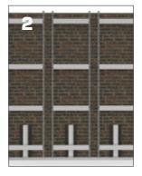
2. Place the steel frames for cladding on the profile, align, and attach them to the masonry wall.
