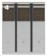
Place the cladding panels up to the height of the connections / fixtures and cut openings for the connections / fixtures.
